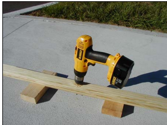
Stack lattice pieces, and drill \frac{1}{4} " holes starting in the center and working your way to the edge with a hole drilled at 12" from the center hole.
